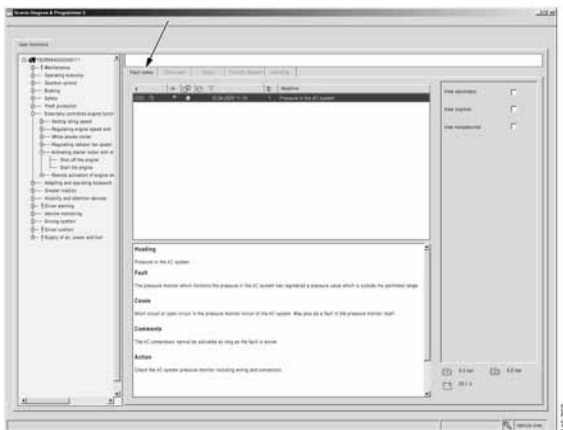
*Fault codes: fault code information for the vehicle is displayed here.*
